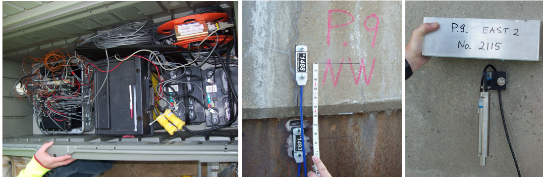
Figure 5. Monitoring system: data logger, strain gage and tiltmeter
