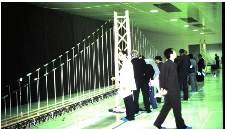
Fig. 14. Aeroelastic Model of Akashi-Kaikyo Bridge (Courtesy of John M. Kulicki)
