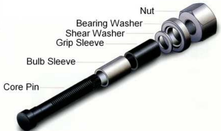
Figure 1 Components of high strength blind bolt
