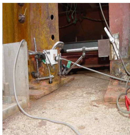
Figure 10. Sensors for measuring girder deflection
